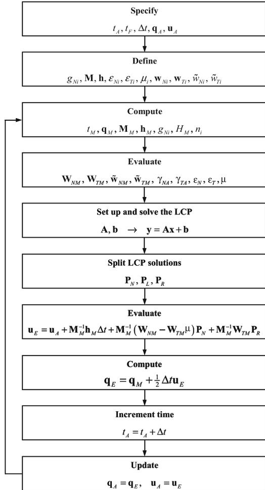
**Fig. 5** Flowchart of the Moreau's time-stepping algorithm with an LCP formulation
