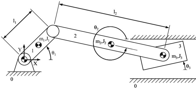
Fig. 6 Slider-crank mechanism with a translational clearance joint
