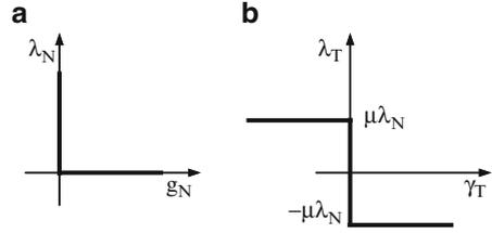
The inequality complementarity behavior of the normal contact law is depicted in Fig. 3a and shows a set-valued graph or a corner of admissible combinations between  $g_N$  and  $\lambda_N$  [22]. When two rigid bodies are contacting, the Signorini's condition given by Eq. (12) needs to be complemented with an impact law, such as the well known Newton's kinematical law that relates the pre- and post-impact velocities to the bodies' normal coefficient of restitution,  $\varepsilon_N$ .
