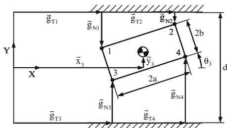
**Fig. 9** Generic position of the slider inside the guide where the distance between guide upper and lower surfaces is exaggerated for illustration purpose
