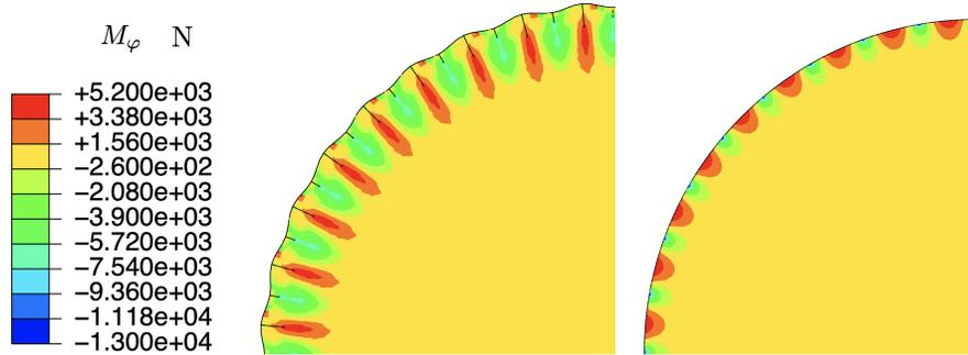
Figure 15: Contour plot of the section moment  $M_\varphi$  for the corrugated-edge dome (left) and for the spherical cap without corrugation (right). In both cases 36 discrete supports have been considered.
