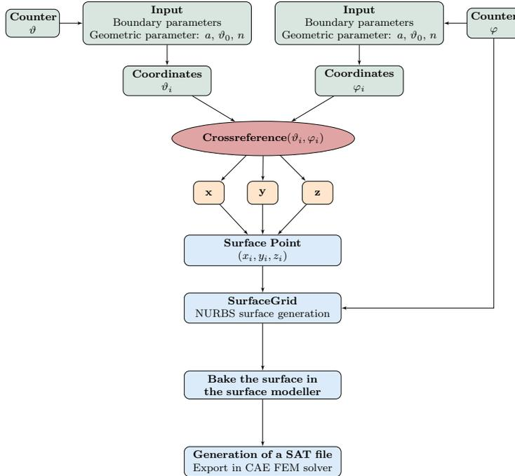
Figure 6: Block-diagram of surface generating algorithm.
