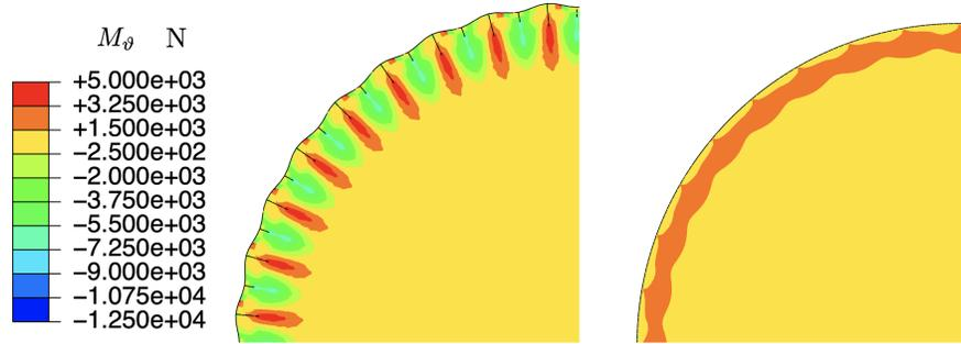
Figure 14: Contour plot of the section moment,  $M_\vartheta$  for the corrugated-edge dome (left) and for the spherical cap without corrugation (right). In both cases 36 discrete supports have been considered.
