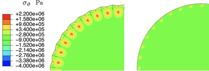
Figure 10: Contour plot of the stress component  $\sigma_{\vartheta}$  for the corrugated-edge dome (left) and for the spherical cap without corrugation (right). In both cases, 36 discrete supports have been considered.
