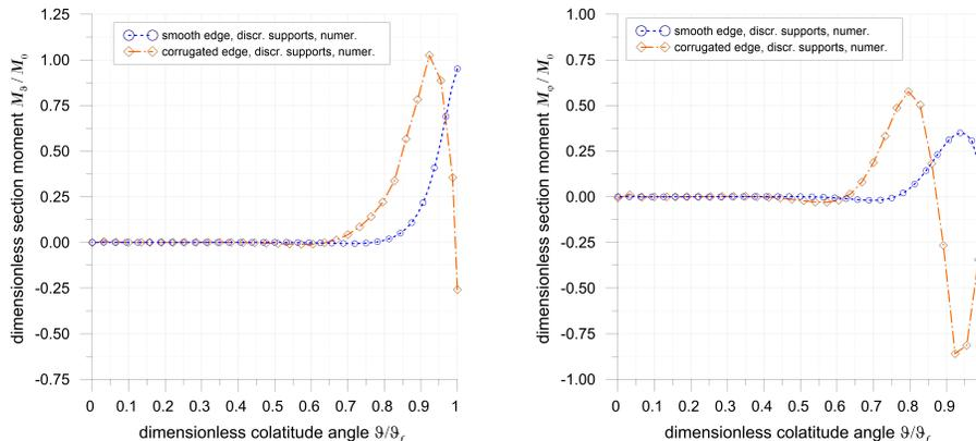
Figure 17: Section moments  $M_\theta$  (left) and  $M_\varphi$  (right) along a meridian located between two supports, i.e. corresponding to the crest of the wave.
