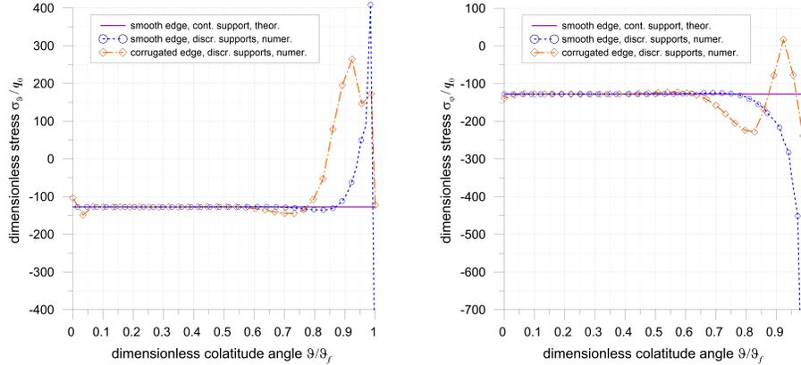
Figure 12: Stress components  $\sigma_\theta$  and  $\sigma_\varphi$  along a meridian passing through a support.
