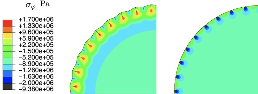
Figure 11: Contour plot of the stress component  $\sigma_\varphi$  for the corrugated-edge dome (left) and for the spherical cap without corrugation (right). In both cases, 36 discrete supports have been considered.
