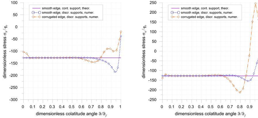
Figure 13: Stress components  $\sigma_\vartheta$  and  $\sigma_\varphi$  along a meridian located between two supports, i.e. corresponding to the crest of the wave.
