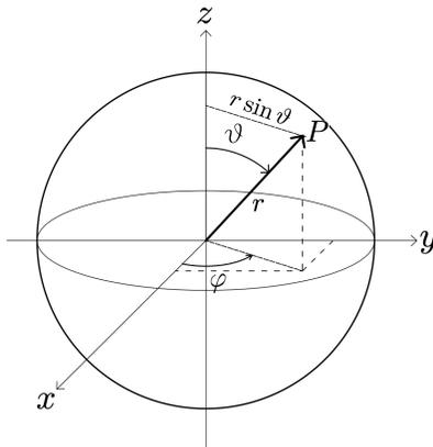
Figure 3: Spherical polar coordinate system.
