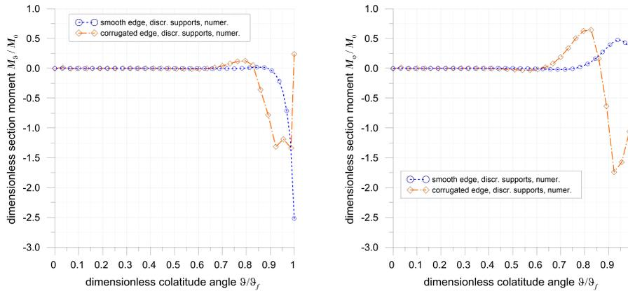
Figure 16: Section moments  $M_\vartheta$  and  $M_\varphi$  along a meridian passing through a support.
