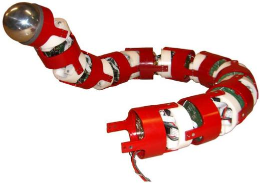
Fig. 1. NTNU/SINTEF snake robot “Aiko.”
