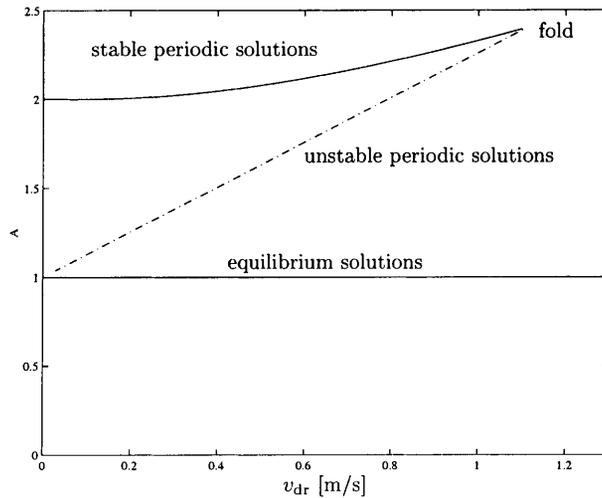
Fig. 7. Bifurcation diagram of the block-on-belt model
