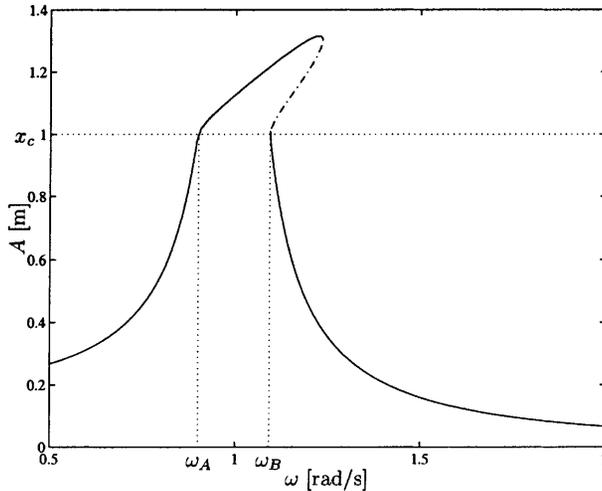
Fig. 3. Response diagram of trilinear spring system
