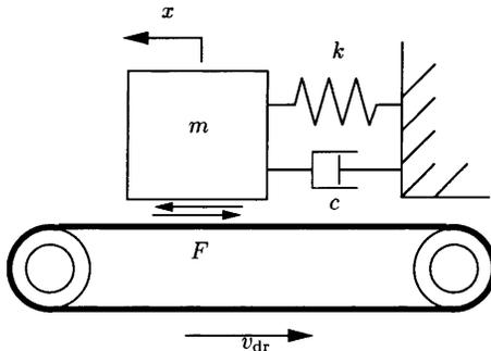
Fig. 5. 1-DOF model with dry friction
