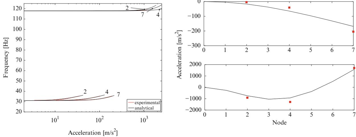
**Fig. 20.8** *Left:* Comparison of first harmonic of frequency-amplitude dependence of analytical and experimental. *Right:* Comparison of the mode shapes for the measured nodes 2, 4, 7 with the analytical mode shape (*top:* mode 1 at 34.5 Hz, *bottom:* mode 2 at 118.5 Hz)
