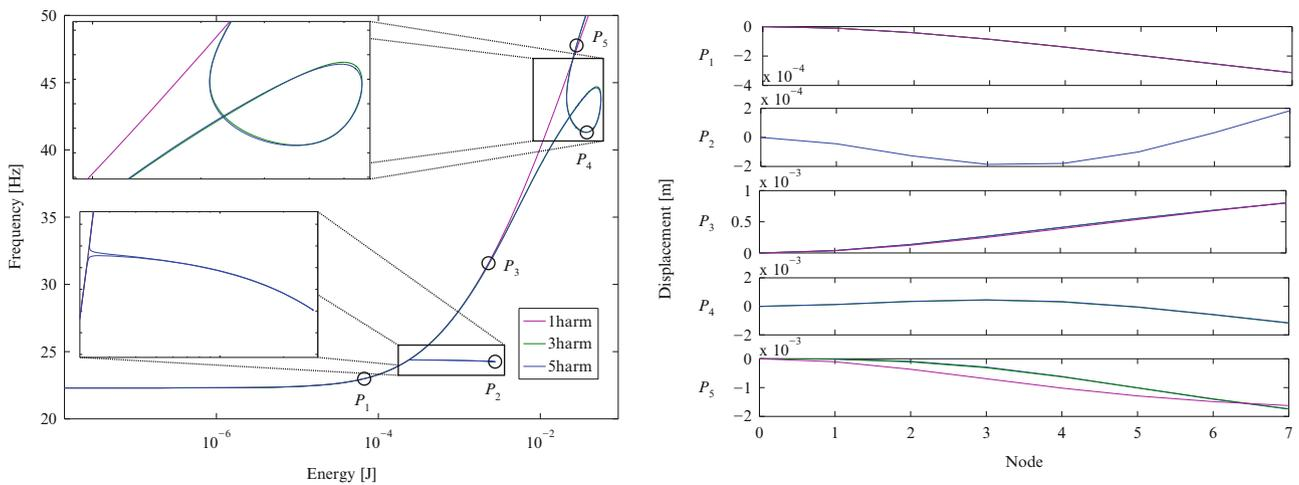
**Fig. 20.2** Left: Filtering of HBM with different number of harmonics for the first mode of a beam with cubic nonlinearity. Right: Comparison of the mode shapes for the points P1 to P5 with different numbers of harmonics
