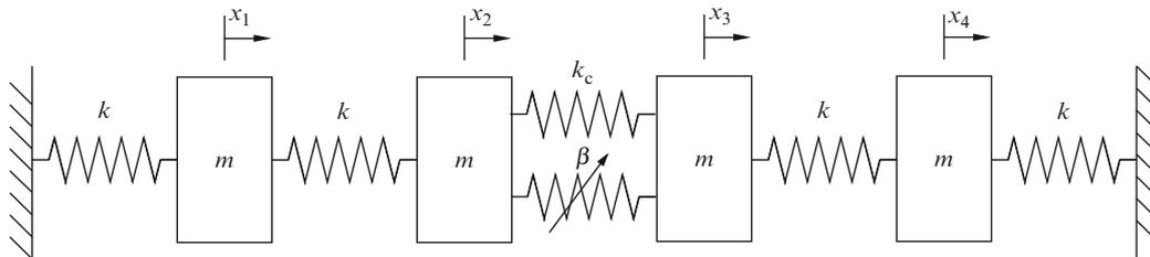
**Fig. 20.3** 4DOF system with cubic coupling element
