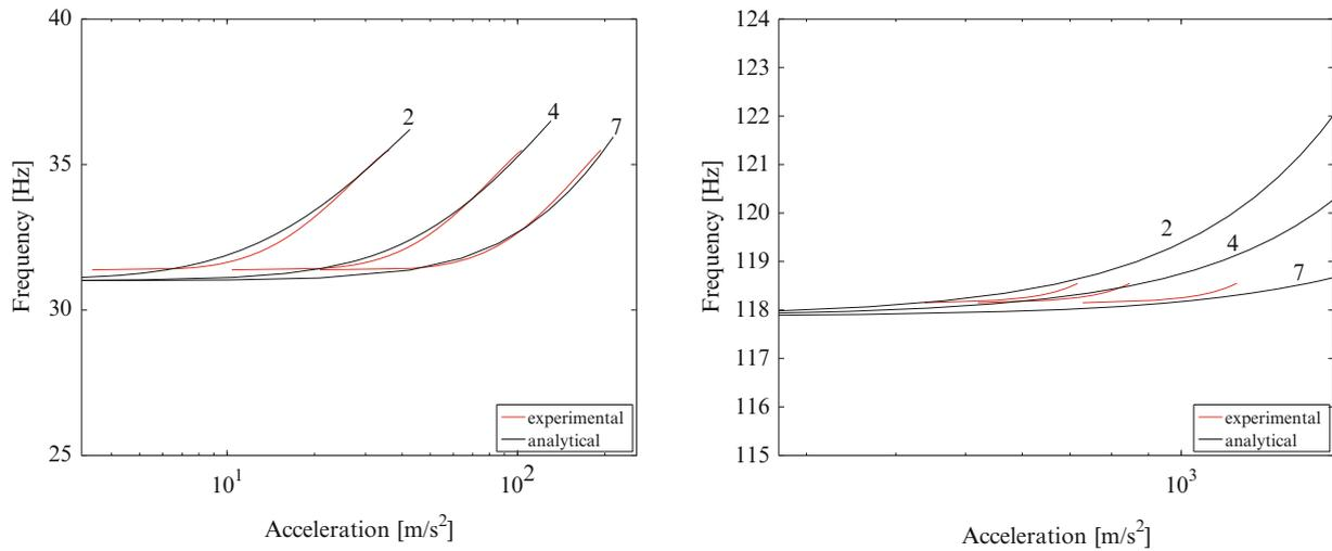
**Fig. 20.9** *Left:* Zoom on the frequency-amplitude dependence curve of first NNM for points 2, 4 and 7. *Right:* Zoom on the frequency-amplitude dependence curve of second NNM for points 2, 4 and 7
