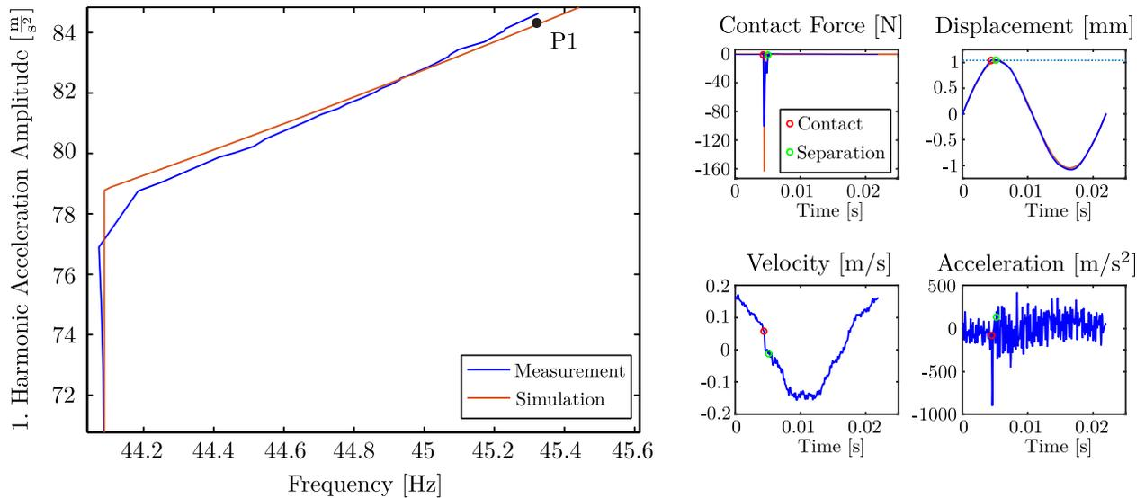
Figure 2: Left: Experimental and numerical backbone curve for the beam tip. Right: Comparison of contact force and displacement (top) and measured velocity and acceleration (bottom) for point P1.
