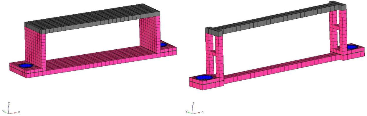
Figure 2: FE models with 6936 and 3468 DOFs used for algorithms testing
