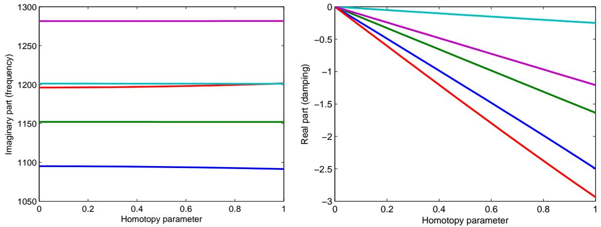
Figure 3: Imaginary and real part of five eigenvalues of the 164 DOF model
