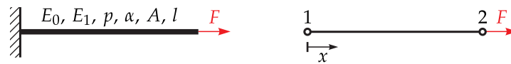
Figure 7. Fractional viscoelastic rod (left) described as a two-node one-dimensional finite element (right).
