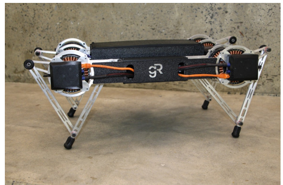
Minitaur: robot with a five-bar mechanism for foot placement
