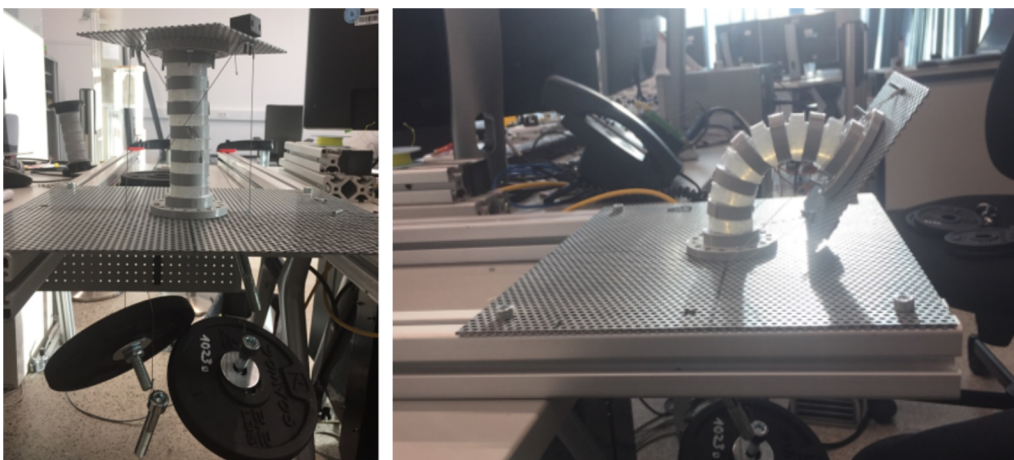
Figure 1: Compliant tendon-driven platform actuated by weights.
