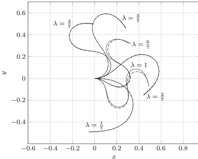
**Fig. 10.9** Deformed configurations of the different beam models under a non-conservative follower force with load parameters  $\lambda \in \{\frac{1}{7}, \frac{2}{7}, \frac{3}{7}, \frac{4}{7}, \frac{6}{7}, 1\}$ . The Timoshenko beam model is depicted by solid lines, the Euler–Bernoulli beam by dashed lines and the inextensible Euler–Bernoulli beam model by dashdotted lines.
