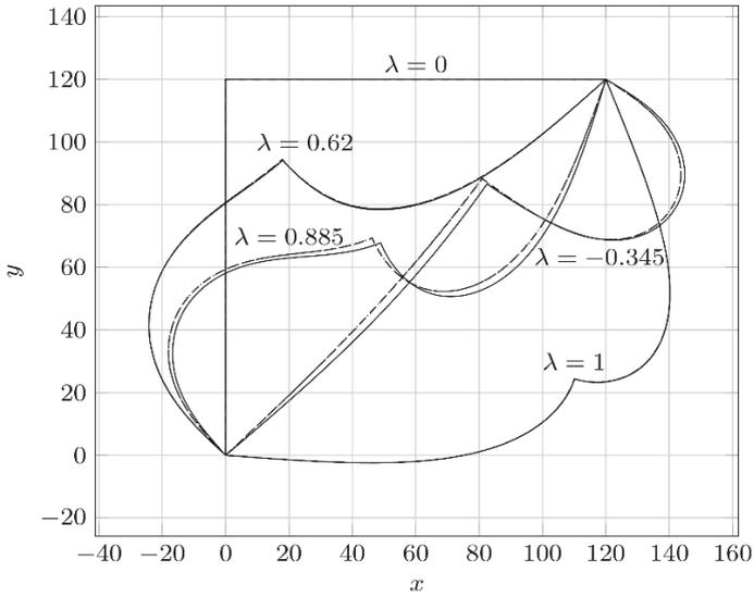
**Fig. 10.13** Deformed configurations of the different beam models for load parameters  $\lambda \in \{0, 0.62, 0.885, -0.345, 1\}$ . The Timoshenko beam model is depicted by solid lines, the Euler–Bernoulli beam by dashed lines and the inextensible Euler–Bernoulli beam model by dashdotted lines.
