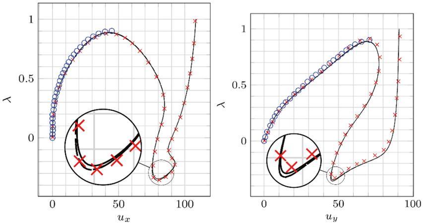
**Fig. 10.14** Load deflection curves of the point of applied force for the horizontal displacement  $u_x = x(L_2) - 120$  and the vertical displacement  $u_y = -(y(L_2) - 120)$ . The Timoshenko beam model is depicted by solid lines, the Euler–Bernoulli beam by dashed lines and the inextensible Euler–Bernoulli beam model by dashdotted lines. The results of Argyris and Symeonidis (1981) are depicted by blue circles, the ones reported by Simo and Vu-Quoc (1986) using red crosses.
