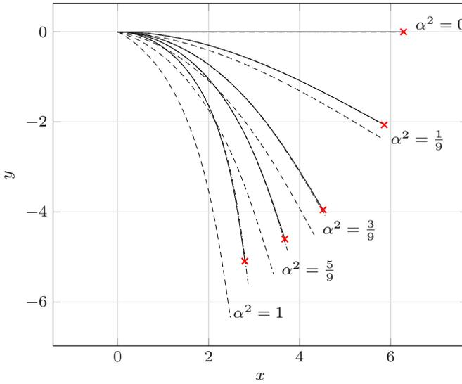
**Fig. 10.7** Configurations for different load parameters  $\alpha^2 \in \{0, \frac{1}{9}, \frac{3}{9}, \frac{5}{9}, 1\}$ . The Timoshenko beam is depicted by dashed lines, the Euler–Bernoulli beam by dashdotted lines and the inextensible Euler–Bernoulli beam model by solid lines. The elliptic integral solutions given in Bisshopp and Drucker (1945) are indicated by red crosses.
