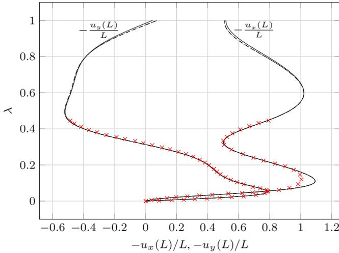
**Fig. 10.10** Load deflection curves for the horizontal displacement  $u_x = x(L) - L$  and vertical displacement  $u_y = -y(L)$  of the point of applied load. The Timoshenko beam model is depicted by solid lines, the Euler–Bernoulli beam with dashed lines and the inextensible Euler–Bernoulli beam model by dashdotted lines. The results found in Argyris and Symeonidis (1981) are depicted by red crosses.
