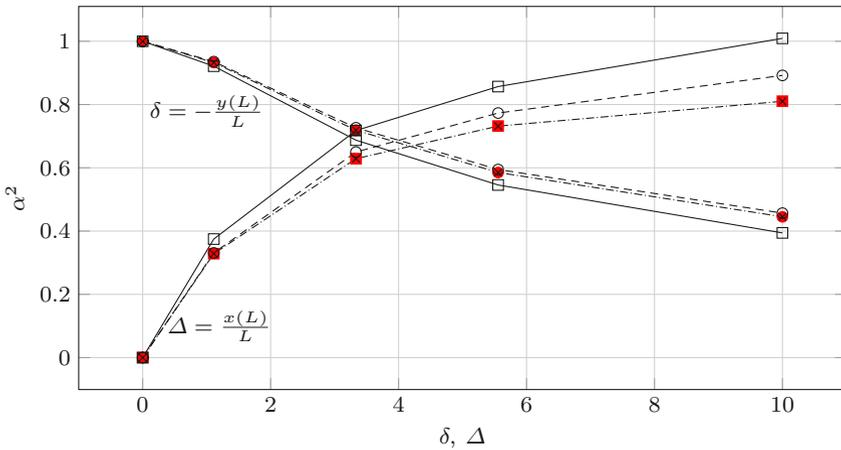
**Fig. 10.8** Force displacement curves for the cantilever beam. The analytical solutions using elliptic integrals are depicted by red bullets and squares for the  $\delta$  and  $\Delta$  values, respectively. The finite element solutions of the Timoshenko beam are depicted by solid lines, the Euler–Bernoulli beam by dashed lines and the inextensible Euler–Bernoulli beam model by dashdotted lines.
