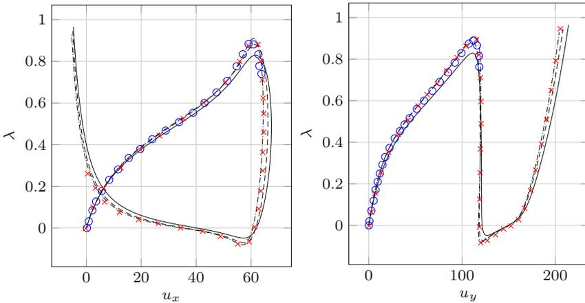
**Fig. 10.12** Load deflection curves for the horizontal displacement  $u_x = x(L_1)$  and vertical displacement  $u_y = -(y(L_1) - 100)$  of the point of applied load. The Timoshenko beam model is depicted by solid lines, the Euler–Bernoulli beam by dashed lines and the inextensible Euler–Bernoulli beam model by dashdotted lines. The results of Dadeppo and Schmidt (1975) are depicted by blue circles, the ones computed by Simo and Vu-Quoc (1986) by red crosses.
