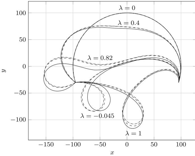
**Fig. 10.11** Deformed configurations of the different beam models for load parameters  $\lambda \in \{0, 0.4, 0.82, -0.045, 1\}$ . The Timoshenko beam model is depicted by solid lines, the Euler–Bernoulli beam by dashed lines and the inextensible Euler–Bernoulli beam model by dashdotted lines.
