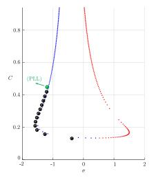
Fig. 5: Backbone curve for r = 0.65. The green point represents the starting point attained with the PLL for G = 1.1. The black crossed circles correspond to the estimated values from the free resonant response.
