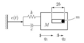
Fig. 1: Scheme of a LO coupled with a vibro-impact absorber (LO-VI NES).
